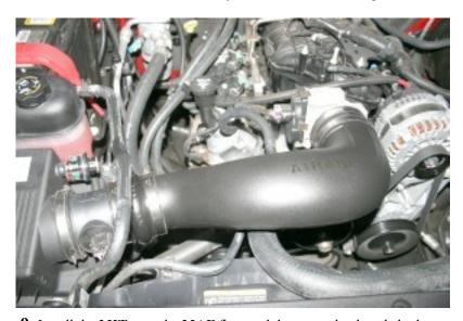
**9.** Install the **MIT** onto the **MAF** first, and then onto the throttle body. Adjust for fit, and tighten the hose clamps. Next connect the breather hose to the factory breather port on the valve cover. Reinstall the factory hose clamp barb back into the hole in the bottom of the **MIT**. Reinstall the beauty cover.
