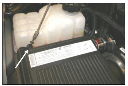
**7.** If you purchased the 200-996 kit, proceed to step # 9. If you purchased the 200-796 Jr. Kit, remove 4 screws in the factory airbox with a #25 Torx bit, and remove the factory air filter. Proceed to step #8.
