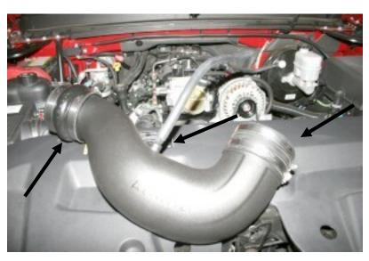
**6.** Install the urethane coupler (#4) on the throttle body end of the Modular Intake Tube (#2) with two #64 hose clamps (#6). Install the urethane hump hose (#3) on the other end of the MIT with the remaining two #64 hose clamps. Leave all clamps loose for now. Install the 3/8" barbed fitting (#7) into the MIT, and slide the 3/8" breather hose (#5) over the barbed fitting as shown.
