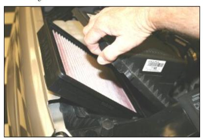
**8.** Install the Airaid Premium filter (#1) into the factory airbox, and reinstall the 4 screws.
