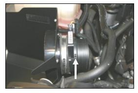
**10.** Re-install the Mass Air Flow sensor onto the filter adapter, and tighten the hose clamp. Make sure the rectangle area where the wiring connects is pointing straight up.
