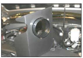
**8.** Install the filter adapter (#5) into the **CAD** using three button head bolts (#9), and washers (#10)
