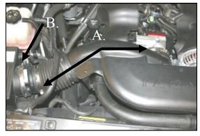
**2.** A.) Loosen the hose clamps on both ends of the factory intake tube. B.) Next loosen the hose clamp on the Mass Air Flow sensor where it clamps on the factory airbox.
