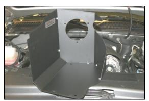
7. Assemble the two Cool Air Dam panels (#2) and (#3) using the five supplied screws (#12), washers (#13), and nuts (#14), as shown.
