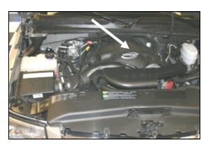
1. **Disconnect negative battery cable.** With a 5/16" socket, remove one bolt on the top of the beauty cover. Set the bolt and the cover aside for re-installation later.
