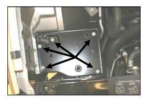
**6.** Remove 5 bolts and remove the factory airbox mounting plate.
