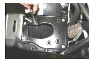
**6.** Using a 10mm socket, remove 5 bolts from the factory airbox mounting plate. Remove the plate from the vehicle.
