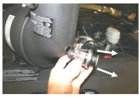
**5.** Remove the factory filter minder and grommet from the factory airbox. Save them for later use.
