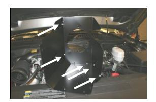
7. Assemble the two Cool Air Dam (CAD) panels (#2) and (#3) as shown, using the five 6-32 screws (#10), washers (#11), and nuts (#12).
