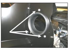
**8.** Install the Airaid intake tube (#4) into the Cool Air Dam using the three 1/4"-20x1/2" button head bolts (#6), and washers (#7) as shown.
