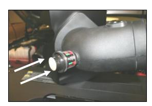
**9.** Re-install the factory grommet and filter minder removed in step #5 into the Airaid intake tube.
