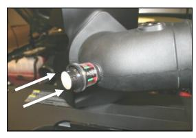
**9.** Re-install the factory grommet and filter minder removed in step #5 into the Airaid intake
