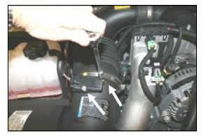
2. Using a #20 Torx bit, remove 2 screws holding the Mass Air Flow sensor to the factory airbox tube.
