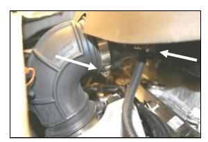
2. Loosen the hose clamp that holds the rubber elbow to the factory air cleaner housing. Next squeeze the tab on the Mass Air Flow sensor wiring connector, and remove the connector from the Mass Air Flow sensor.
