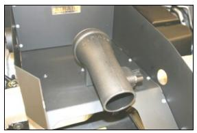
**10.** Install the Airaid Intake Tube onto the **CAD** using two  $1/4-20 \times 1/2$ " button head bolts (#7) and 1/4" flat washers (#8), threaded up from the bottom of the **CAD**.
