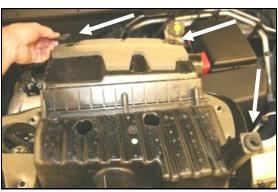
**5.** Remove 3 factory rubber grommets from the factory air cleaner housing.
