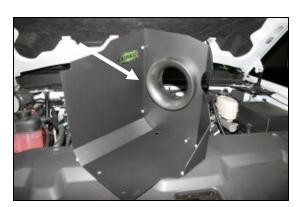
**8.** Assemble the Cool Air Dam panels (CAD) (#2 & #3) using five 6-32 x 5/16" screws (#10), #6 flat washers (#11), and 6-32 keps nuts (#12). Next install the air filter adapter (#5) into the panels as shown using three 1/4 - 20 x 1/2" button head bolts (#13), and 1/4" flat washers (#14).
