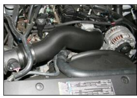
**12.** Install the Airaid Intake Tube into the hump hose first, and then onto the throttle body. Adjust it for fit, and then tighten the hose clamps.
