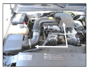
1. Disconnect the negative battery cable. Loosen the hose clamps on each end of the factory intake tube assembly and remove tube.
