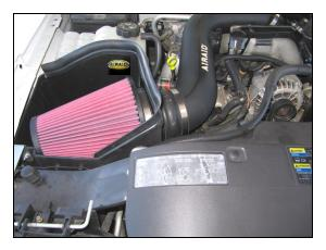
15. Install the Airaid Premium Filter (#1) onto the filter adapter, and tighten the hose clamp. Install the weather strip (#7) onto the Airaid Cold Air Box. Reconnect the M.A.F. sensor . (Note: Start from one corner and work your way around to insure proper alignment of the weather strip.)
