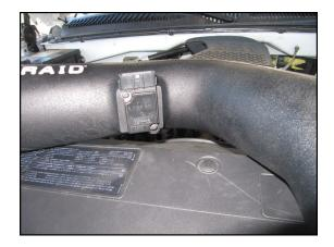
8. Transfer the M.A.F. Sensor from the factory airbox into the Airaid intake tube (#2). Use the two 8-32 button head screws (#10). to secure the meter.
