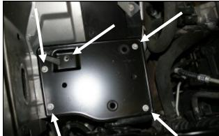
5. Using a 10mm socket, remove the bolts that secure the factory air filter housing platform and remove it from the vehicle.
