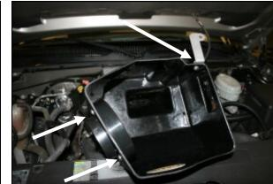
6. Install the filter adapter (#4) into the Cool Air Box (#3) as shown using three 1/4" Button head bolts (#8) and three 1/4" flat washers (#11). Next, fasten the bracket to the front of the **CAB** as shown using one 1/4-20 hex bolt (#9) two flat washers (#10), and one 1/4" Nylock nut. Refer to the drawing above for reference.
