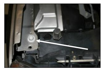
7. Remove the factory bolt that secures the right front fender to the radiator support. It will be reused in step
