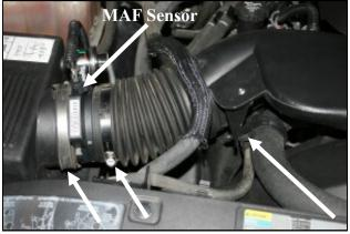
2. Loosen two hose clamps. One on each side of the Mass Air Flow (MAF) sensor. Using a flat blade screwdriver, disconnect the factory intake tube from the plastic clamp on the radiator hose
