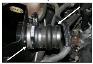
9. Reinstall the MAF sensor and coupler onto the filter adapter and tighten the clamp. Next install the hump hose (#5) onto the MAF using two
