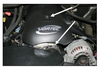
1. <u>Disconnect the negative battery cable.</u> Loosen the bolt that secures the beauty cover to the engine and remove it and the cover from the vehicle. Loosen the hose clamp that secures the factory air intake tube to the throttlebody.
