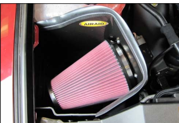
17. Install the Airaid Synthamax Filter onto the Intake Tube inside of the Cold Air Box. Install the Weather Strip onto the top edge of the Cold Air Box with the contour rolling away from the filter.
