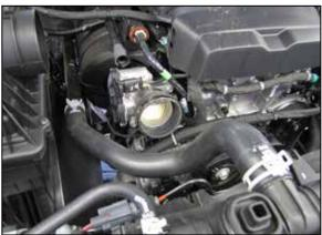
6. Install the provided coupler hose (084036) onto the throttle body and secure with the provided hose clamp.
