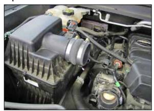
8. Install the provided coupler (08171) onto the air filter housing and secure with the provided hose clamp.
