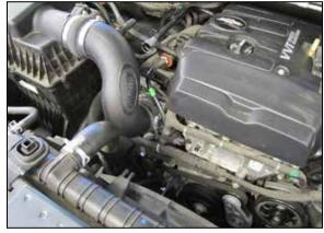
9. Install the intake tube into the coupler at the throttle body, align with the coupler on the air filter housing. Adjust the tube for best fit and secure with the provided hose clamps. Reconnect the mass air sensor electrical connection.
