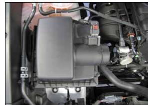
4. Loosen the four bolts that secure the upper air filter housing to the lower housing, remove the housing and factory air filter.
