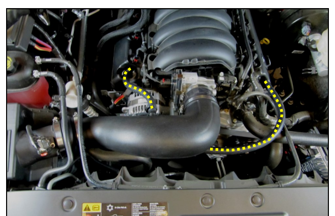
9. Install the Intake Tube and tighten the Clamps. Connect the new breathers to the Barbed Fittings in the Intake tube and the Quick Connect Fittings to the Valve covers.
