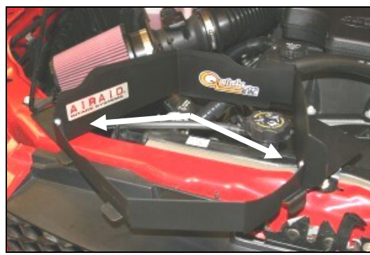
5. Assemble the Quick Fit panels (#2&#3) using the four 6-32x5/16" screws (#5), #6 washers (#7), and nuts (#6).
