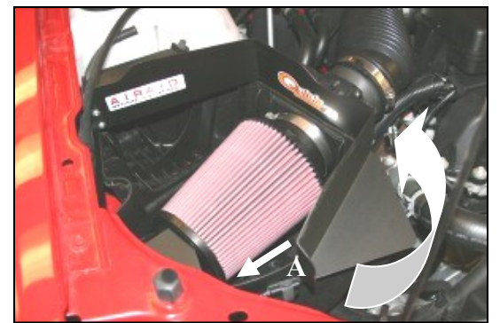
6. Install the Quick Fit panels by inserting the tab on the front of the panel into the front slot of the factory airbox base (A), and then rotating the panels counterclockwise.
