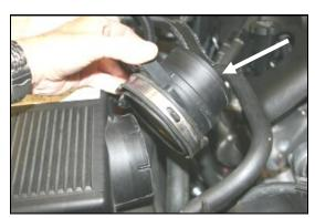
**4.** Without disconnecting the electrical connector, remove the **M**ass **A**ir **F**low sensor from the factory airbox, and set it aside.
