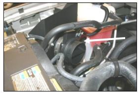
**10.** Re-install the Mass Air Flow sensor onto the filter adapter, and tighten the hose clamp. Make sure the rectangle area next to where the wiring harness connects is pointing up.
