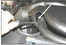
**3.** Using a screwdriver, pry the factory tube away from the plastic clamp on the radiator hose, and remove the tube.
