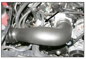
12. Install the Airaid Intake Tube into the hump hose first, and then onto the throttle body. Adjust it for fit, and tighten the hose clamps. Next install the 3/8° x 14° breather hose (#8) between the 1/4° NPT x 3/8° barbed fitting in the tube, and the factory port on the valve cover.
