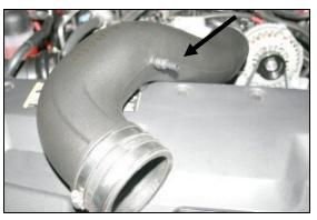
**11.** Install the 1/4" NPT x 3/8" Barb Fitting (#18) into the Airaid Intake Tube as shown. Next install the urethane coupler (#7) onto the throttle body end of the tube using two #64 hose clamps (#17). Tighten *only* the clamp on the tube.
