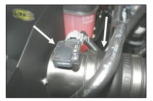
**10.** Reinstall the **MAF** sensor onto the filter adapter using two 8-32 x 5/8" Allen Bolts (#13). **Do Not Use The Factory Screws!** Next install the urethane hump hose (#6) onto the
