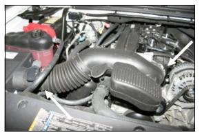
4. Loosen two hose clamps on the factory intake
