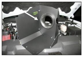
8. Assemble the Cool Air Dam panels (CAD) (#2 & #3) using five 6-32 x 5/16" screws (#10), #6 flat washers (#11), and 6-32 keps nuts (#12). Next install the air filter adapter (#5) into the panels as shown with the hole for the Mass Air Flow sensor facing up, using three  $1/4 - 20 \times 1/2$ " button head bolts (#14), and 1/4" flat washers (#15).
