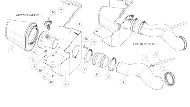
4. Loosen two hose clamps on the factory intake tube. One at the throttlebody, and one where it clamps to the factory airbox. Remove the factory intake tube from the vehicle.
