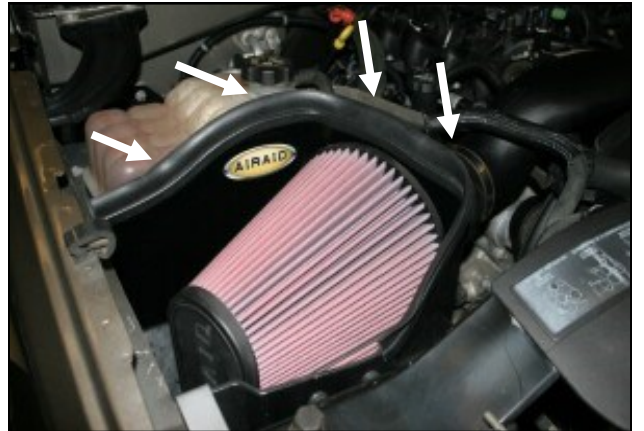
12. Install the provided weather strip (#7) along the top edge of the Airaid Cool Air Dam starting at the right fender working your way around towards the radiator. Install the Airaid Premium Filter (#1) onto the air filter adapter and tighten the hose clamp. Reinstall the factory beauty cover removed in step #1.. Double check your work!
