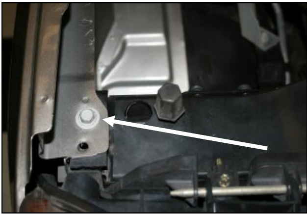
7. Remove the factory bolt that secures the right front fender to the radiator support. It will be reused in step #8.
