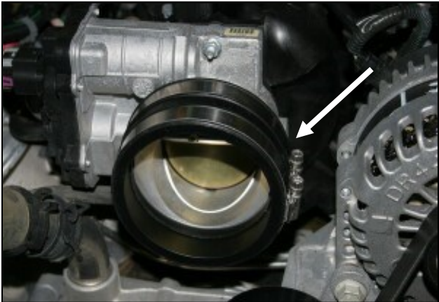
10. Install the provided coupler (#6) with two #64 hose clamps (#14) onto the throttle body. Do not tighten the clamps at this time.
