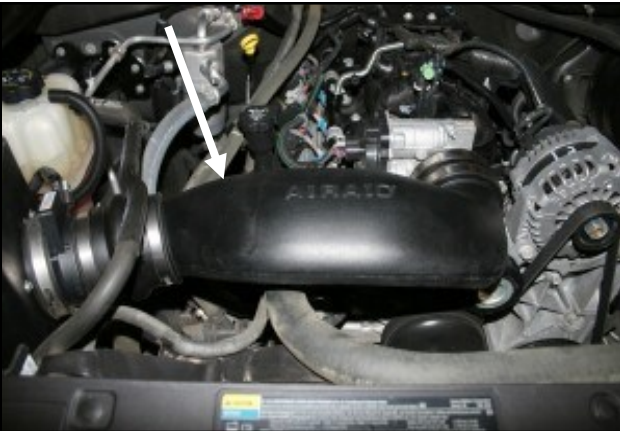
11. Install the small end of the intake tube into the hump hose first and then rotate it slightly to slide the other end into coupler on the throttlebody. Adjust for fit, and then tighten all four hose clamps.
