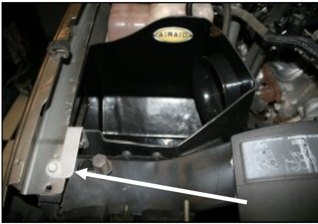
8. Install the CAB assembly into the vehicle where the factory airbox used to be using three 6mm hex bolts (#12) and three flat washers (#11) thru the bottom. Now reinstall the factory fender bolt thru the bracket and into the fender. Adjust the assembly for fit and tighten all bolts and nuts at this time.
