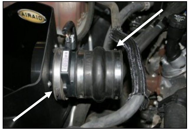
9. Reinstall the MAF sensor and coupler onto the filter adapter and tighten the clamp. Next install the hump hose (#5) onto the MAF using two #60 hose clamps (#13). Leave these two clamps loose for now.
