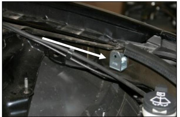
12. Replace the ground lug from step #11 with the side bracket (#25) as shown using one 6mmx12mm hex bolt (#14), and lock washer (#12).
