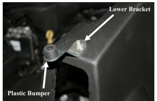
**9.** Turn the CAB upside down and mount the lower bracket (#26) to the bottom of the CAB using one 1/4-20x3/4" hex bolt (#10), 1/4" flat washer (#11), and 1/4" Nylock nut (#13) as shown. Next using one 8-32x5/8" button head screw (#17), and one #8 Kep nut (#18), attach the plastic bumper (#19) to the bracket as shown.
