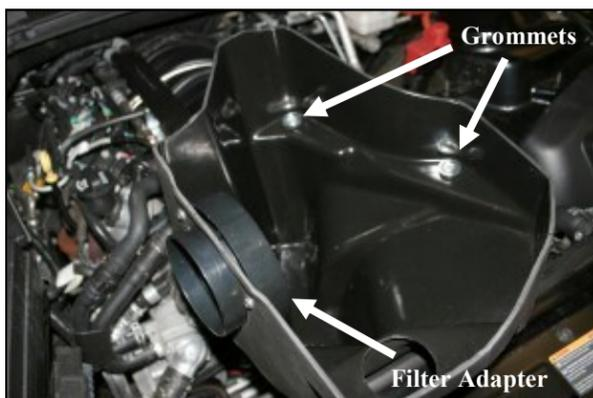
**8.** Reinstall the two steel sleeves and grommets into the Airaid Cold Air Box (CAB) (#3). Next install the filter adapter (#4) into the CAB as shown using three 1/4-20x3/4" hex bolt (#10), 1/4" flat washer (#11), and 1/4" Nylock nut (#13) as shown. Next using one 8-32x5/8" button head screw (#17), and one #8 Kep nut (#18), attach the plastic bumper (#19) to the bracket as shown.
