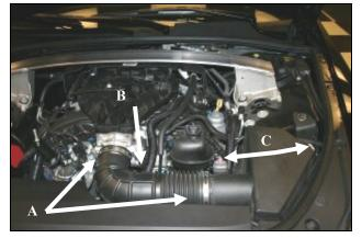
2. A) Loosen the hose clamps on the factory intake tube. **B**) Disconnect the breather line and remove the factory intake tube . C) Disconnect the Mass Air Flow and MAP sensors.
