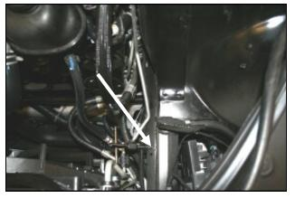
5. Locate the pre existing hole in the chassis and tap it for a 1/4-20 bolt. Use a 1/4-20 NC tap with anti-seize lube or equivalent, and follow the 1/4 turn forward, 1/2
