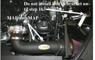
**13.** Install the Airaid Intake Tube assembly onto the filter adapter first, and then onto the throttle body. Adjust for fit, and tighten all the hose clamps. Next, reconnect the **MAF** and **MAP** sensors.
