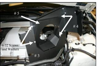
6. Install the Adapter Panel (#5) to the MAF Panel (#3) as shown using four 6-32 screws (#12), 6-32 Kep nuts,
