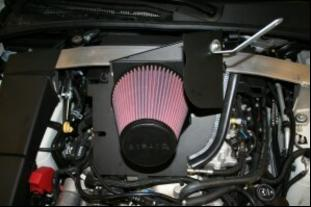
**11.** Install the Bracket (#28) on to the Rear Panel (#3) as shown using one 1/4-20 Button Head Screw (#17), 1/4" Flat Washer (#20), and 1/4" Serrated Nut(#21). Complete the assembly by attaching the Airaid Premium Filter (#1) to the Filter Adapter (#10).
