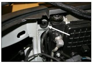
**4.** Use caution not to loose the factory core support grommet while removing the air box assembly. It will be
