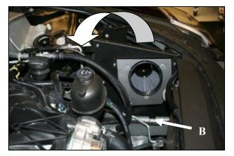
**12. A)** Lower the Airaid Performance Air box assembly into the engine cavity . Insert the Well Nut into the Factory core support grommet and rotate the assembly rearward until the bracket rests on the shock tower and the MAF panel's lower tab hole is lined up with the Tapped Chassis bolt hole from step **5**. **B)** Secure the assembly by using the 1/4-20x 3/4 Bolt(#19).
