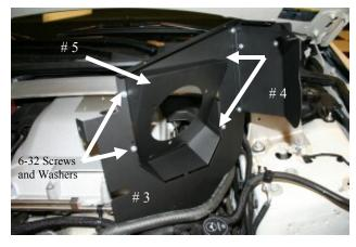
**6.** Install the Adapter Panel (#5) to the MAF Panel (#3) as shown using four 6-32 screws (#12), 6-32 Kep nuts, and #6 flat washers (#14). Attach the Rear Panel (#4) to the MAF Panel using two 6-32 screws.
