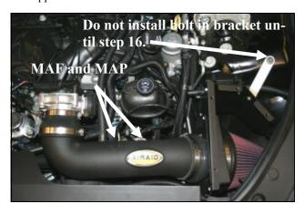
**13.** Install the Airaid Intake Tube assembly onto the filter adapter first, and then onto the throttle body. Adjust for fit, and tighten all the hose clamps. Next, reconnect the **MAF** and **MAP** sensors.
