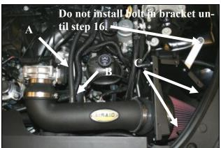
**14. A)** Replace the factory breather line on the valve cover with the 26" Airaid Breather Hose(#12). **B)** Secure the breather hose to the intake tube nipple using the black Speed Clamp (#32).C) Slide the Edge Clip Cable Ties (#31) about 6" apart along the fender pinch weld and return the coolant line to it's original location. Secure the coolant line using the cable ties and trim off excess.
