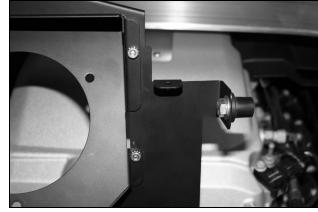
**8.** Attach the 5/8" Well Nut (#25) to the vertical MAF Panel tab as shown using the 5/16 Hex Bolt (#23) and the 5/16" flat washer (#24).
