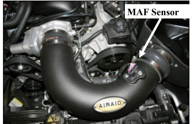
15. Install the Airaid Intake Tube (#2) into the hump hose first, and then into the reducing coupler. Adjust for fit, and tighten all four hose clamps. Next install the MAF sensor into the tube and secure it using two 8-32 x 3/8" button head screws (#20).
