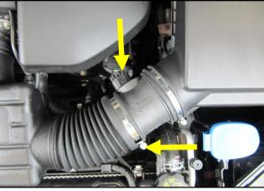
**2.** Disconnect the Mass Air Flow sensor and loosen the intake tube clamp.
