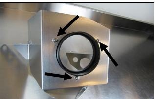
**4.** Separate the intake tube from the Mass Air Flow sensor and remove the entire air box assembly from the vehicle.
