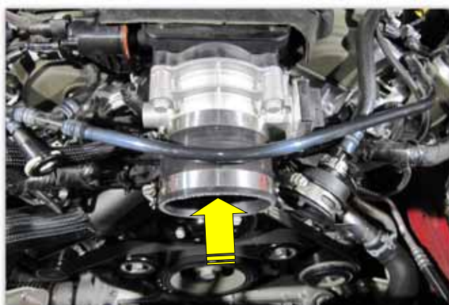
20. Slide the Coupler and #48 Clamps onto the throttle body as shown.
