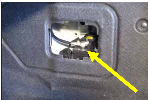
1. Inside the trunk, on the passenger side, locate and remove the battery access panel. Disconnect the Negative battery terminal.
