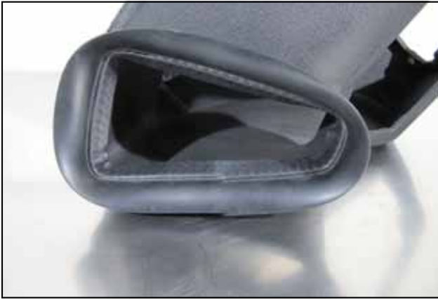
13. Install Weatherstrip onto the Airbox inlet, with the contour flaring out. Trim any excess for a proper fit.
