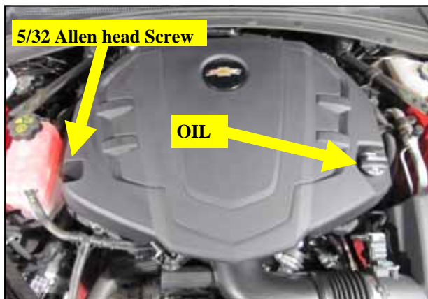
2. Remove the oil cap and engine cover. Reinstall the oil cap for the remainder of the install.
