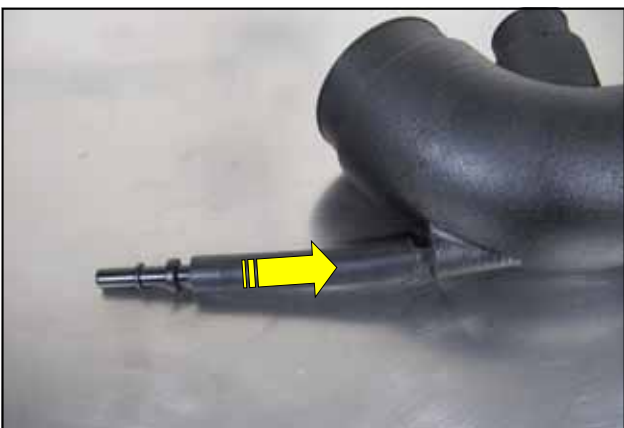
16. Insert the PCV fitting into the supplied Hose and connect it to the Barbed Fitting on the Tube.
