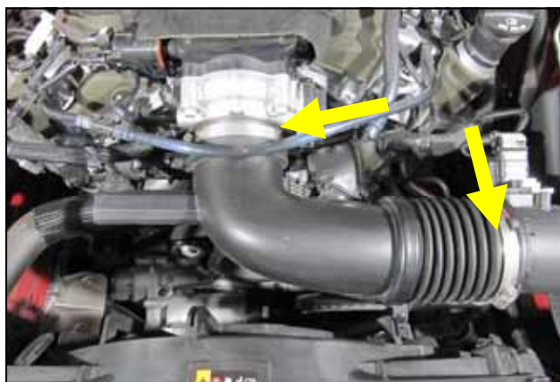
4. Loosen the clamps on the intake tube and remove it from the vehicle.
