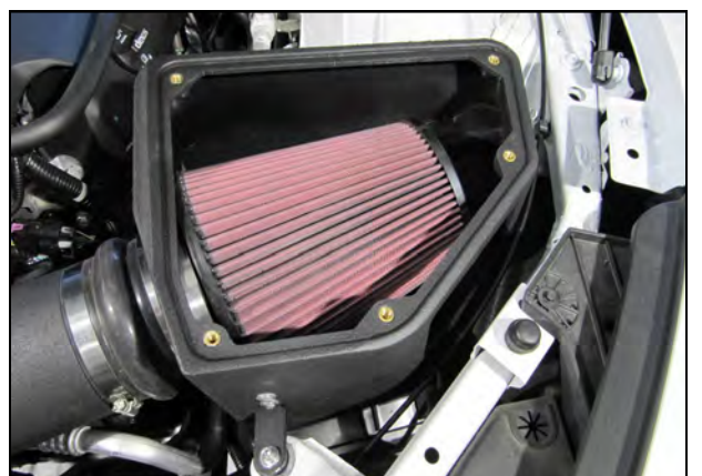
23. Install the Airaid Premium Airfilter on to the Filter Adapter in the Airbox.
