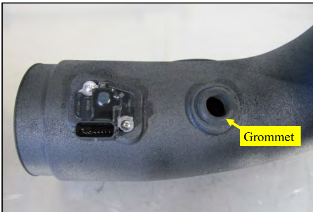
14. Transfer the MAF Sensor from the factory airbox, into the Airaid Intake Tube and secure it using the supplied #8 Button Head Screws. Insert the Grommet into the Intake Tube as shown.
