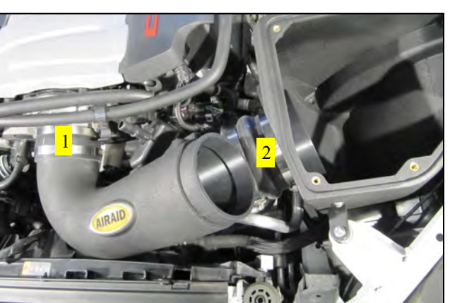
21. Insert the Intake Tube into the Coupler first, then into the Hump Hose.
