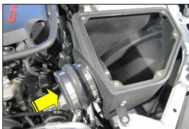
19. Slide the Hump Hose and #72 Clamps onto the Filter Adapter.
