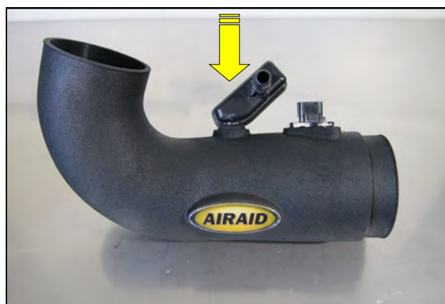
16. Transfer the PCV fitting into the Grommet in the Airaid Intake Tube. Apply the Airaid Badge to the Intake Tube as shown.
