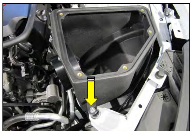
17. Place the Airaid Airbox assembly into the engine compartment as shown, with the mounting posts only fully seated in all three grommets.
