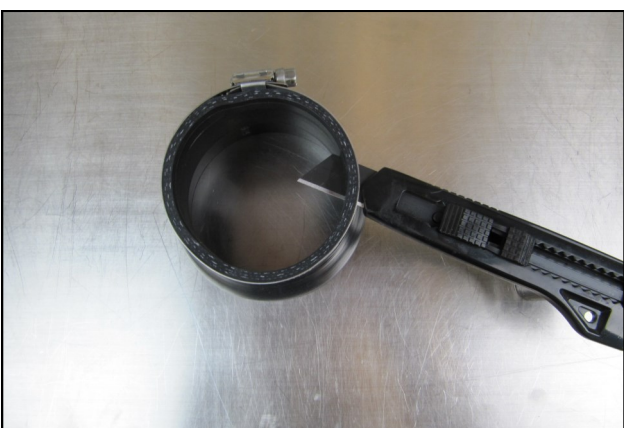
7. Using a utility knife or equivalent, trim the Coupler in one single pass. HINT: Keep the blade tight against the clamp while cutting and deeply inserted into the Coupler for a clean cut.
