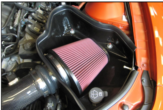
19. Install the Airaid Premium Filter (#1) onto the Filter Adapter and tighten the clamp. Next install the Weather Strip (#7) onto the top of the CAB. For ease of installation, start the front of the CAB near the radiator and work your way around towards the fender
