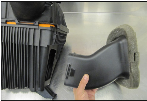
10. Compress the sides of the factory intake scoop and remove it from the airbox.
