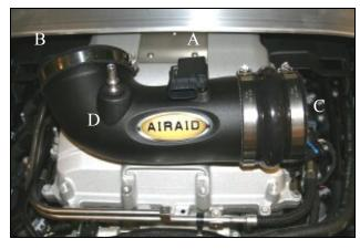
9. A) Transfer the Mass Air Flow sensor from the Factory airbox assembly into the Airaid Intake Tube(#2). Secure to the tube by using the 8-32 screws (#15) and #8 lock washers (#16). B) Install the GM Coupler (#9) on to throttle body side of the intake tube. C) Install the Hump Hose (#10) on the filter side of the intake tube as shown. D) Insert the Grommet (#24) into the hole in the Airaid Intake Tube and then follow by inserting the barbed end of the PCV Fitting (#25) into the Grommet.
