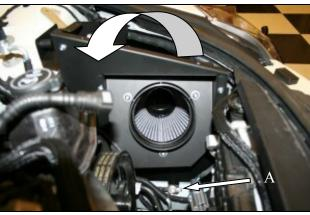
11. A) Locate and remove the Factory Ground strap bolt in the chassis. B) Lower the Airaid Performance Airbox assembly into the engine cavity. Insert the Well Nut into the Factory core support grommet and rotate the assembly rearward until the bracket rests on the shock tower and the MAF panel's lower tab hole is lined up with the Chassis bolt hole. Secure the assembly by reusing the factory 6mm Chassis Bolt.
