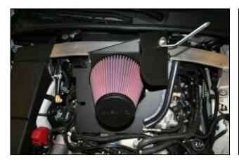
**10.** Install the Bracket (#27) on to the Rear Panel (#4) as shown using one 1/4-20 Button Head Screw (#19), 1/4" Flat Washer (#18), and 1/4" Serrated Nut(#20). Complete the assembly by attaching the Airaid Premium Filter (#1) to the Filter adapter (#8).
