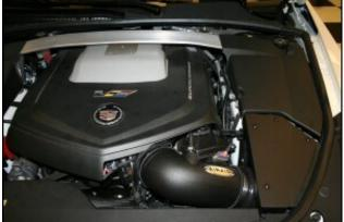
**14.** Reinstall the Factory engine and shock tower covers.
