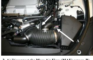
**2. A)** Disconnect the Mass Air Flow (MAF) sensor. **B)** Disconnect the PCV breather line by depressing the 2 Grey buttons in the fitting and pulling. Loosen the clamps securing the intake tube to the throttle body and airbox and remove the factory intake tube.
