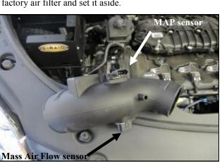
7. Transfer the air sensors from the factory airbox lid into the Airaid Intake Tube(#2) as shown. **Do Not Use**The Factory Hardware. Secure the Mass Air Flow sensor using the two #8-32 screws (#16), and the MAP sensor using the 1/4-20x 3/4 hex head bolt (#9) and 1/4" Flat Washer (#12).
