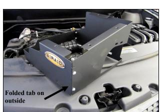
**5.** Join the two Airaid panels together with the folded tabs on the **outside**, using the four 6-32 screws (#15), #6 Flat washers (#14), and #6 Keps Nuts (#13).
