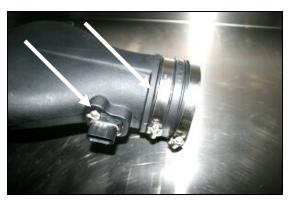
**9.** Reinstall the Mass Air Flow sensor removed in step #5, into the Airaid Intake Tube using two 8-32x3/8" button head bolts (#7).
