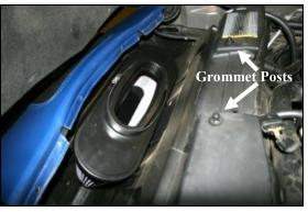
11. Set the Airaid Premium Filter into the area in front of the radiator. It will be mounted in step # 15
