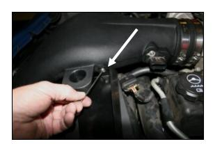
**14.** Tighten all four button head bolts that retain the air dams to the intake tube, and the radiator shroud
