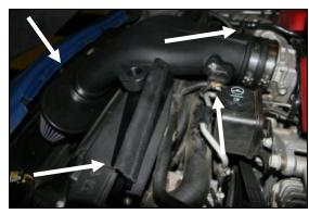
15. Slide the Airaid Premium Filter up onto the end of the intake tube and tighten the clamp. Reconnect the MAF sensor wiring harness and replace the grey security clip. Reconnect the factory breather hose to the breather fitting. Install the weather strip (#6) onto the top of the air dams as shown.
