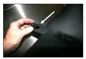
**8.** Install the two factory grommets that were removed in step #4, into the Airaid Intake Tube as shown
