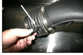
**6.** Remove the factory breather fitting from the factory intake tube and save for reinstallation in step #7.
