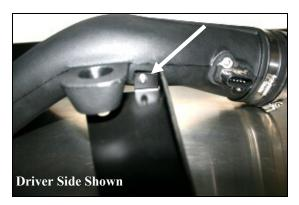
**10.** Attach the two air dams (#4 driver side & #5 passenger side) onto the Airaid Intake Tube using one 8-32x1/4" button head bolt (#8) and #8 flat washer (#9) on each side. Leave the bolts slightly loose for now to allow for adjustment.
