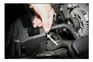
13. Slide one clip nut (#10) over the outside end of the plastic radiator cover and align it with the hole in the air dam. Install one rubber washer (#11) over the threads of the clip nut, and then align the air dam hole over the washer. Add one more rubber washer, one #8 flat washer (#9), and one M4 Pan Head Screw (#8) to secure the air dam. Repeat this step on the passenger side. Refer to the line drawing on page one.
