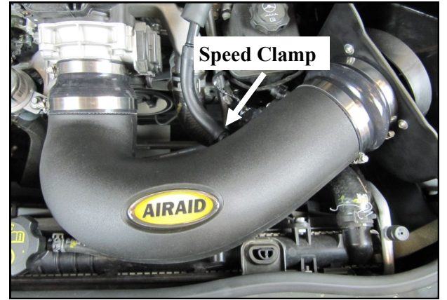
15. Install the Airaid Intake Tube into the hump hose first, and then into the coupler. Adjust for fit, and tighten all four Hose Clamps. Reconnect the PCV breather using the supplied PCV Hose. Slide the hose onto the factory hard line and onto the Intake Tube's Barbed Fitting. Use the Speed Clamp (#13) to secure the Hose onto the Fitting. Reconnect the Mass Air Flow meter.
