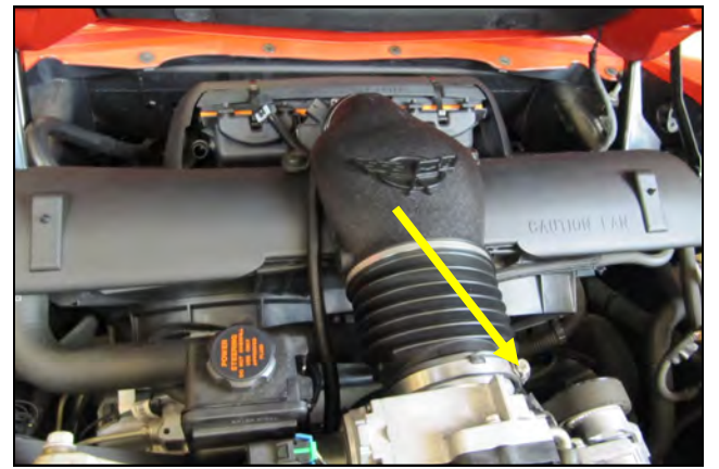
3. Loosen the intake tube clamp on the throttle body.
