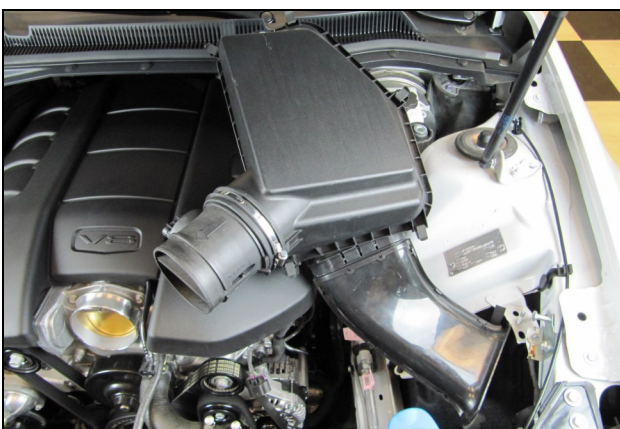
4. Remove the entire air box assembly from the vehicle.
