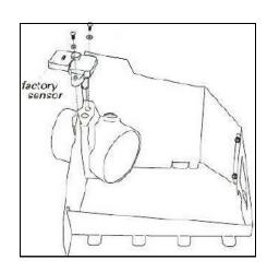
**10.** Install the factory **IAT** sensor into the air filter adapter using two 8-32 button head screws (#12), and #8 flat washers (#13).
