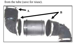
**4.** A.) Loosen the hose clamp that secures the factory airbox lid to the intake tube assembly, and remove the assembly from the lid.
