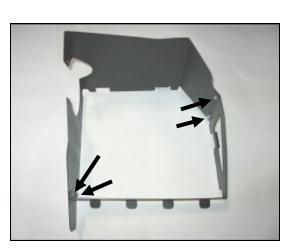
**8.** Assemble the Airaid Cool Air Dam (CAD) panels (#2, #3) using four 6-32x 5/16" screws (#7), #6 flat washers (#8) and 6-32 keps nuts (#0)
