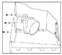
**9.** Mount the air filter adapter (#5) onto the **CAD**, using three 1/4-20x 5/8" hex bolts (#10), and three 1/4" flat washers (#11).
