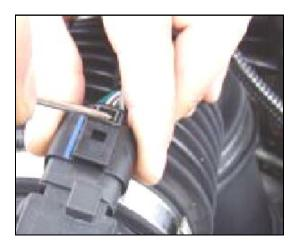
**13.** Reconnect the **IAT** sensor wiring harness to the sensor.
