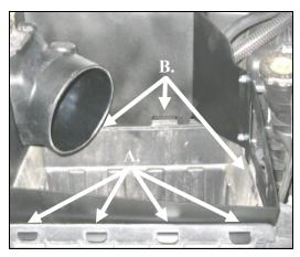
11. A.) Install the **CAD** by inserting the four tabs into the side of the factory airbox.
