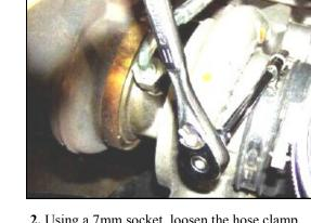
**2.** Using a 7mm socket, loosen the hose clamp where the factory intake tube connects to the turbo housing.
