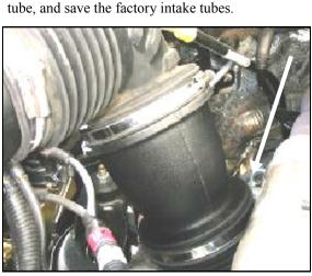
**7.** Install the Airaid Intake Tube assembly onto the turbocharger inlet. Tighten the factory hose clamp.
