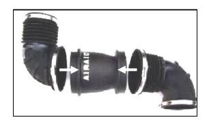
**5.** Replace the factory silencer tube with the Airaid Intake tube (#4). Complete the Airaid Intake tube assembly by aligning the notches in the tubes, and tightening the factory hose clamps.
