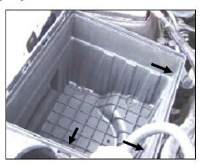
**3.** Unlatch the three clips on the factory air box. Remove the factory intake tube assembly and airbox lid from the vehicle.
