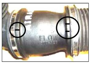
**6.** Note: Each side of the Airaid Intake Tube has notches that must be aligned with the notches on the factory intake tubes. Also, the flow arrow must point down towards the turbocharger inlet.
