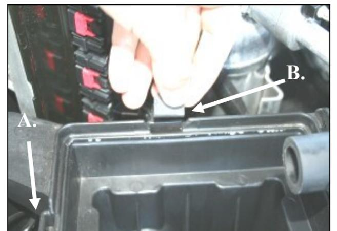
4. **2007 and newer models only:** A.) Using a flat blade screwdriver, gently pry and remove one factory clip from the passenger side rear of the airbox base. (see arrow above)
