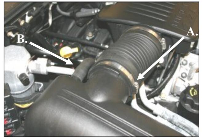
2. A.) Loosen the hose clamp on the factory airbox lid.
