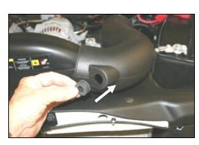
**8.** Install the grommet (#11) into the Airaid Intake Tube (#3).
