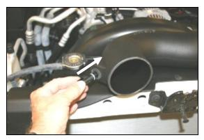
**10.** Carefully install the **AIT** sensor into the grommet in the Airaid Intake Tube. Make sure it goes all the way in.
