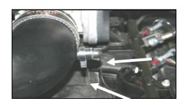
**12.** Install the provided rubber cap (#7) and speed clamp (#10) onto the nipple on the Modular Intake Tube, as shown.
