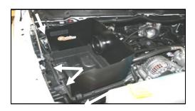
**8.** Install the Quick Fit Panel (#2) onto the factory airbox base by sliding the tabs on the base thru the Quick Fit Panel and then adjust the sides to fit. Re-latch the 4 clips to hold the Quick Fit
