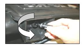
**6.** Gently twist the air temperature sensor counterclockwise and remove it from the
