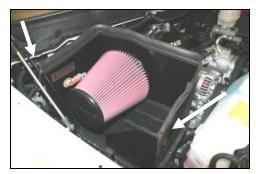
**14.** Install the Airaid Premium Filter (#1) onto the tube on the Quick Fit Panel and tighten the clamp. Next install the weather strip (#6) on the top of the Quick Fit Panel as shown. (*Hint: Start at one end of the Quick Fit Panel and work your way towards the other end.)*
