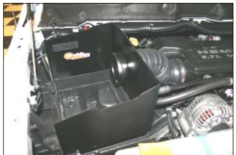
4. Install the Cool Air Dam (#2) by slipping it into the factory intake tube, and then sliding it over the tabs on the factory airbox base. Adjust it for fit on top of the airbox base, and re-latch the 4 clips to hold the CAD securely in place.
