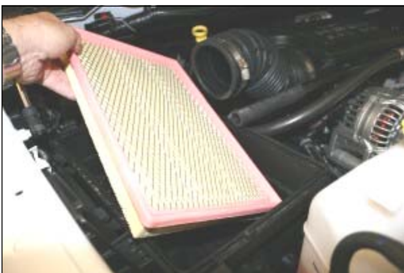
3. Remove the factory air cleaner.
