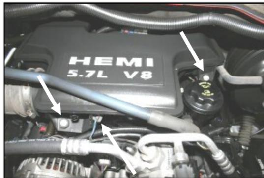
**2.** Squeeze the tab on the connector and disconnect the intake temperature sensor wiring harness on the front of the resonator. Next remove the two bolts that secure the resonator to the engine. Lift the resonator up at the front, and remove it from the vehicle.
