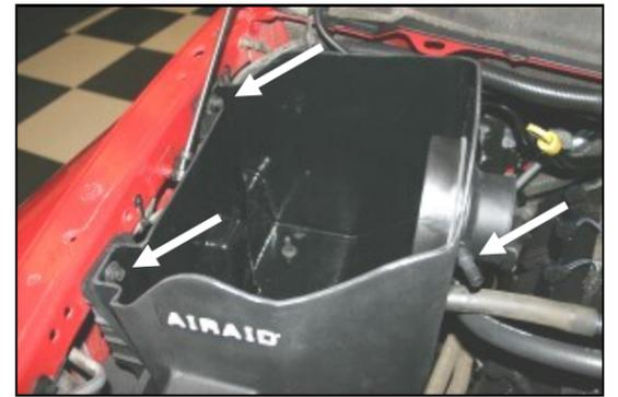
**9.** Install the CAD into the vehicle by aligning the grommets over the locating pins on the factory airbox mount. Reinstall the factory bolts in the fender that were removed in step #4. Next install the 1/4"NPT x 1/2" barbed fitting (#19) into the CAD.
