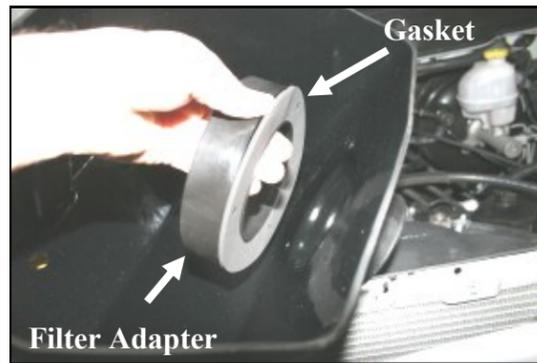
**8.** Install the adapter gasket (#25) and filter adapter (#6) into the CAD using three 1/4-20 x 5/8" bolts (#8) and flat washers (#9) as shown. Refer to the line drawing above for reference.
