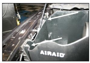
**9.** Install the **CAB** into the vehicle by aligning the grommets over the locating pins on the factory airbox mount. Reinstall the factory bolts into the fender that were removed in step #3.
