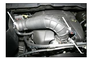
**13.** Reinstall the factory air intake tube. Reconnect the electrical connector to the temperature sensor, and then tighten both hose clamps.
