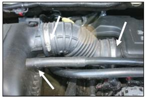
1. **Disconnect the negative battery cable!**Loosen the two hose clamps on the flexible intake tube, one at the airbox lid and one at the resonator. Slide the flexible tube off of the lid and the resonator and remove it from the vehicle.
