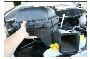
**2.** Rock the airbox back and forth as you are lifting it straight up to remove it from the vehicle. It is only held in by grommets.
