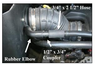
**10.** Install the supplied 3/4" x 2 1/2" hose (#11) onto the factory crankcase breather tube, and then insert the 1/2" x 3/4" barbed connector (#9) into the 3/4" hose. Next connect the 1/2" rubber elbow (#7) from the 1/2" barbed fitting on the filter adapter to the 1/2" x 3/4" connector. See the line drawing on the front page for reference.
