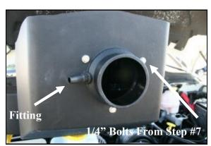
7. Install the 1/4" NPT x 1/2" barbed fitting (#8) into the filter adapter as shown.
