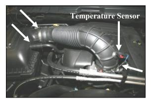
1. **Disconnect the negative battery cable!**Locate the temperature sensor on the air intake tube, slide the red tab, squeeze the black tab on the electrical connector, and then disconnect the temperature sensor from the air intake tube. Disconnect the crankcase breather tube from the air filter box. Loosen one hose clamp at each end of the air intake tube and remove it from the vehicle.
