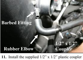
11. Install the supplied 1/2" x 1/2" plastic coupler (#11) into the 1/2" hose from step #10. Next connect the 1/2" rubber elbow (#8) between the 1/2" connector and the barbed fitting on the filter adapter.
