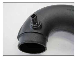
12. Install the inlet air temperature sensor into the AIRAID® intake tube using the provided grommet.
