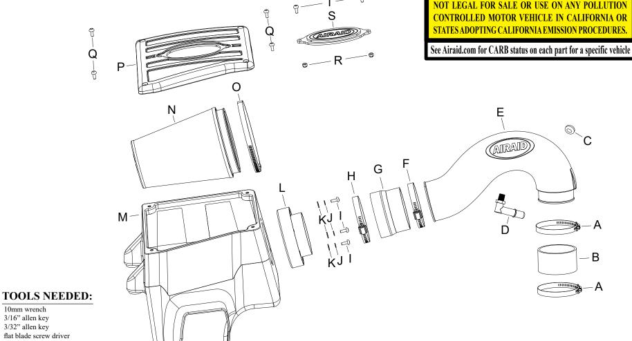
10mm wrench 3/16" allen key 3/32" allen key flat blade screw driver
