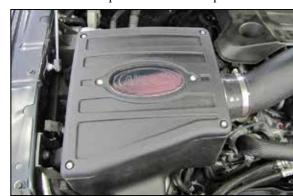
16. Install the AIRAID® window into the air filter housing lid and then install the lid onto the air filter housing and secure with the provided hardware.
