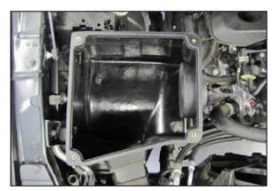
7. Set the AIRAID® air filter housing into the vehicle so that the mounting grommets engage onto the mounting posts.
