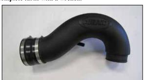
10. Install the provided coupler (KITRDCR30) onto the AIRAID® intake tube and secure with the provided hose clamp.
