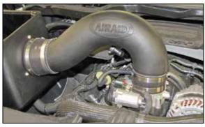
13. Install the AIRAID® intake tube onto the filter adapter and then into the coupler at the throttle body, adjust the tube for best fit and then secure with the provided hose clamps.
