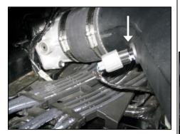
**10.** Reconnect electrical connector on factory air temperature sensor.
