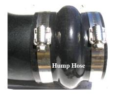
**8.** Install the hump hose and coupler provided onto the Airaid MIT with the supplied hose clamps. The straight coupler is positioned on the throttle body end and the hump hose is positioned on the air filter end.
