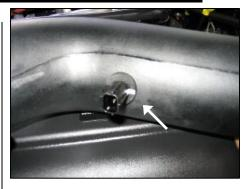
7. Install the supplied grommet and factory air temperature sensor into the Airaid MIT.
