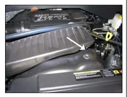
**2.** Unsnap factory air box tube baffle from fan shroud and remove air tube assembly from vehicle.
