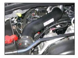
**9.** Check for any foreign objects or debris it the intake path & install Airaid MIT assembly on engine. (<u>Note</u>: Leave hose clamps loose until final assembly)
