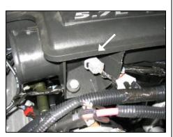
**3.** Carefully disconnect electrical connector from air temperature sensor in factory housing.
