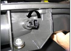
**5.** Remove air temperature sensor from housing by turning counter clockwise and pull.
