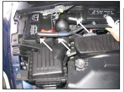
1. Disconnect negative battery cable. Remove valve cover breather hose from air box lid. Loosen hose clamps on both sides of factory intake tube.
