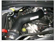
**9.** Install Airaid intake tube assembly by connecting the Airaid hump hose onto the factory air box lid and the other end onto the Airaid reducer hose. Tighten all hose clamps.
