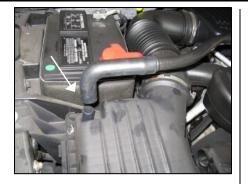
**1.** Disconnect the negative battery cable and remove the breather hose from the factory air box lid.
