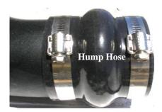
8. Slide the urethane hump hose onto straight end of Airaid intake tube with two #60 hose clamps. (<u>Note</u>: Leave hose clamps loose until final assembly).
