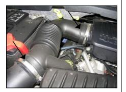
**2.** Loosen the two hose clamps on each end of the factory intake tube.
