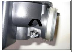
6. Turn the air temperature sensor <sup>1</sup>/<sub>4</sub> turn and remove from the air box. Retain sensor for later use.
