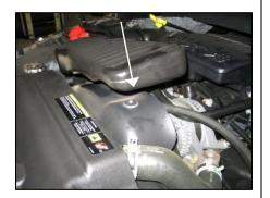
**3.** Unsnap the factory silencer box from the fan shroud and remove the factory tube assembly from the vehicle.
