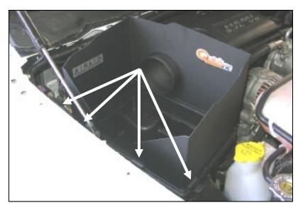
**3.** Position the Airaid Cool Air Dam (CAD) (#2) onto the factory airbox base. Relatch the factory clips onto the CAD.
