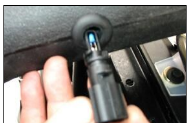
9. 2003-2005 Models Only: Install rubber grommet w/thru hole and insert the factory air temperature sensor into the grommet.
