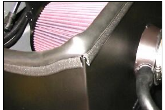
18. 2004-05 Models Only: Connect the factory breather hose to the Airaid Cool Air Dam & secure using the #24 Speed clamp provided.
