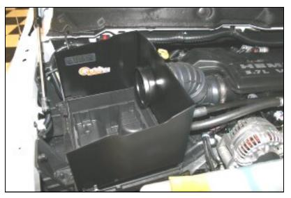
4. Install the Quick Fit Panel (#2) by slipping it into the factory intake tube, and then sliding it over the tabs on the factory airbox base. Adjust it for fit on top of the airbox base, and re-latch the 4 clips to hold the Quick Fit Panel securely in place.
