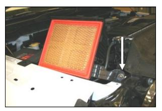
**2.** Using a 10 mm socket, remove the nut that secures the factory airbox, lower half, to the radiator support. Rock the factory airbox assembly side to side to release it from it's mounting grommets, and remove it from the vehicle.
