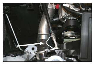
**4.** Remove the two Factory Airbox grommets and set aside. They will not be reused.
