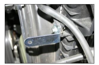
**6.** Install the L-bracket (#20) onto the radiator shroud using one M8 x 30mm bolt (#14) and one flat washer (#12) as shown. Leave the bolt slightly loose for now.
