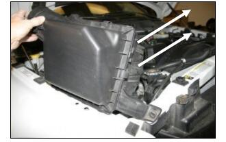
**2.** Slide the flexible intake tube off of the factory airbox lid and then rock the factory airbox assembly side to side to release it from the mounting grommets, and remove it from the vehicle.
