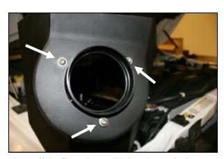
**8.** Install the filter adapter (#4) into the Cool Air Box (#3) using three 1/4" Button Head bolts (#9) and flat washers (#10) as shown.
