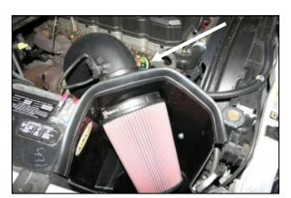
12. Install the Airaid Premium Filter (#1) onto the filter adapter and tighten the clamp. Install the weatherstrip onto the top of the CAB starting at the right fender and working your way towards the radiator. Next reinstall the factory filter minder and grommet into the Airaid Intake Tube.
