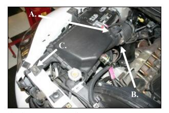
Disconnect the negative battery cables.
