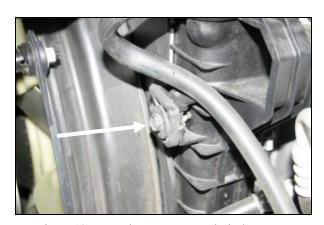
**5.** Using a 13mm socket remove one bolt that secures the fan shroud to the radiator on the passenger side of the vehicle.
