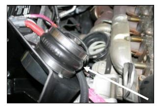
**10.** Install the supplied hump hose (#5) onto the filter adapter using two #72 hose clamps. Leave the clamps loose for now.
