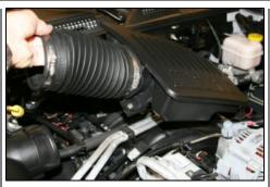
**4.** Remove the resonator and tube from the vehicle.
