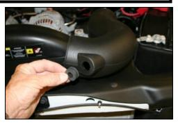
7. Install the grommet into the hole in the MIT as shown.
