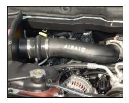
15. Slide the Airaid tube with hump hose into the Airaid Cool Air Dam first, and then slide the other end into the throttle body coupler. (Note: The Airaid tube should be flush against throttle body with a gap between the tube and Cool Air Dam assembly for engine movement.) After inspection, adjust the Airaid tube, coupler, and hump hose and tighten all hose clamps
