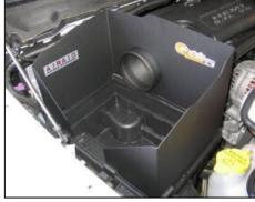
**8.** Position the Airaid Cool Air Dam in place of the original air box lid. Snap in place.
