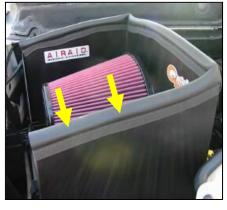
19. Install weather strip along the top rim of the Airaid Intake System. (Hint: start the install at the top corner of the cold air dam)
