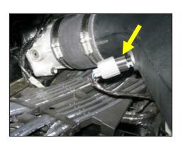
**16.** Re-connect air temperature sensor connector.
