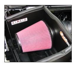
**9.** Mount the Airaid Premium filter inside the Cool Air Dam & secure with hose clamp provided.
