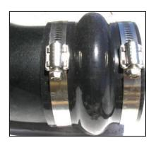
13. Install the urethane hump hose on the long end of the Airaid tube using two of the #60 hose clamps provided. Leave loose for final assembly.
