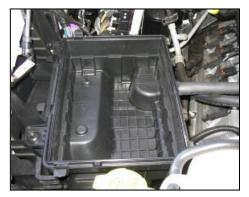
7. Unclip & remove the factory air box lid and factory air filter.
