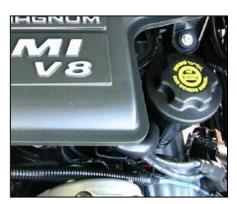
**4.** <u>2003 Models:</u> Disconnect & remove the crankcase vent hose from the front of the factory resonator.
