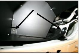
11. Install the CAD assembly into the vehicle, and install the 3/8-16x1 1/4" button head bolt (#18) thru the panel, and into the well nut. Next install the 6x1x12mm hex bolt (#16), and 1/4" flat washer (#12), thru the panel, and into the captured nut in the radiator support. Leave all bolts loose until final adjustment.
