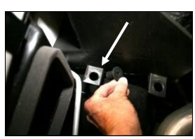
**8.** Install the supplied well nut (#21) into the support bracket hole that is closest to the fender.
