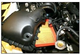
**2.** Unsnap the two metal clips that hold the airbox lid to the base, and remove the lid. Next, remove the factory paper air filter from the base.
