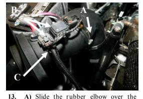
Airaid filter adapter, install one #80 hose clamp (#20), and tighten the hose clamp. **B)** Using three 8-32x1/2" button head screws (#13), reinstall the factory Mass Air Flow sensor, and temperature sensor into the Airaid filter adapter. **Do Not Use The Factory Screws! C)** Reinstall the wiring harness anchor into the hole in the filter adapter just below the temperature sensor.
