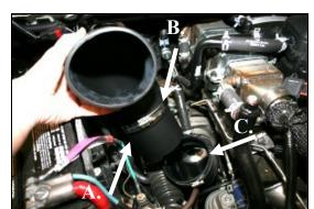
9. A) Install the metal tube (#5) into the rubber elbow (#6) until the rolled bead touches the side. B) Install one #80 hose clamp (#20) around the elbow at the metal tube, and tighten. C) Install the tube assembly into the factory rubber elbow on the turbocharger. Leave the factory hose clamp loose until final adjustments are made.
