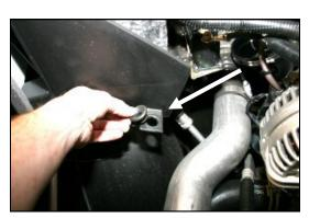
**7.** Remove the two factory rubber grommets that held the factory airbox base in place.
