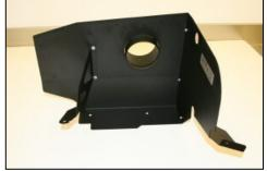
**7.** Assemble the Cool Air Dam as shown using the 5 screws, washers, and nuts provided.
