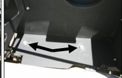
**10.** Install two ½"-20 bolts and washers thru the top, and fender washers and nuts on the bottom, where the factory grommets were removed
