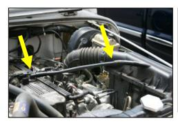
**1.** Disconnect negative battery cable. Remove factory valve cover breather hose from airbox, and valve cover.
