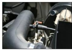
**16.** Slide intake tube into the hump hose first, and then into the coupler. Adjust for a good fit, and tighten hose clamps. Slide vacuum hose on barbed fitting, and install speed clamp as shown.
