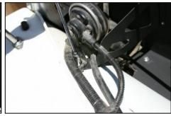
**11.** Slide the CAD bracket under the horn mount and reinstall the factory bolt from step 5.
