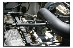
17. Replace the factory breather hose with  $\frac{1}{2}$ "x10" rubber hose between valve cover and intake tube using speed clamps as shown.
